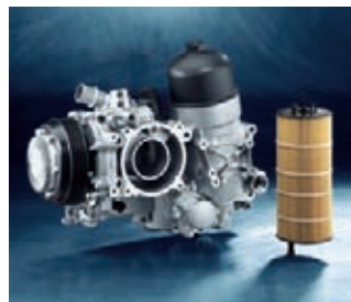
The new MAHLE oil filter module for commercial vehicles is highly versatile in terms of integration on both the oil and coolant side. Thanks to the high level of integration, the number of interfaces and sealing points has been reduced. Both weight and costs have been lowered by employing high-performance plastics.
